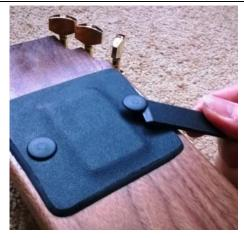
Gently prise out the pins using a flat, blunt(!) blade
