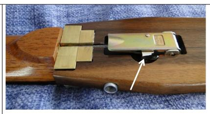
Press the latch on the clamp lever,
