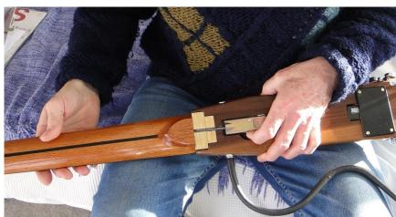
pull the clamp up and rotate it back toward the machine head end of the guitar, disengaging the hook from the tensioning cable.
