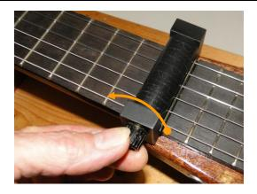
Pull the side clamp off the block to disengage the side pin [1] from the metal hinge block.
